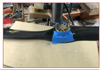
After the first hole is drilled, insert a dowel rod into the first hole. This helps keep the jig from turning on the face of the prop. Using the tape and dowel rod has helped me consistently drill props for years. Note that I use a spill board under my prop while on the drill press.
