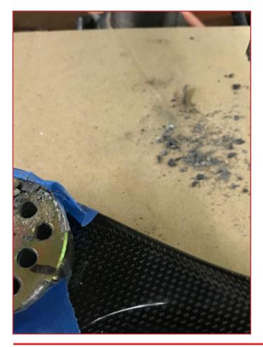
I generally use a small shop vacuum that has a filter to remove this from my drill press area. Once you have drilled all six holes, you should have a cleanly drilled prop. If you find your props split on the opposite side of the prop, use a spill board as I have pictured here and keep in mind you will have to sharpen drill bits more often (or replace) when drilling through carbon fiber.
