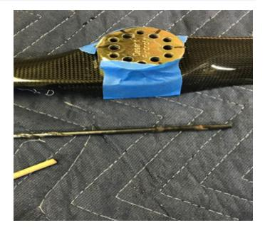
Some modelers will position the holes different depending on their engine starting preference. I usually like my prop to be in the 1 o'clock or 2 o'clock position. Now it's time to start drilling the prop. I will give a note of precaution; in that many of the carbon fiber props and even some wood props, contain very irritating materials and you should always wear protective gloves, eyewear, and a respirator.
