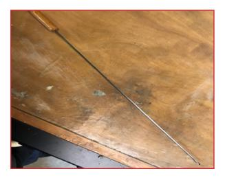
This driver is made from a 1/2" piece of dowel and a 2.5' piece of 1/8" music wire. I first cut a 3" piece of dowel and drill a 1/8" hole about 2.5" into dowel using a drill press. I also carve a notch on the opposite end of the drill hole. I use this notch to tell how far of a turn I'm adjusting my carbs.
