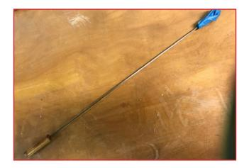
My last tip is for all of you JETI radio pilots out there that use magnetic switches. If your magnetic switch placement cannot be close to the exterior of your plane (i.e. in the canopy a 1/2" or so), you can place one of the neodymium magnets on your magnetic switch key (place magnet near the hole on the key) and you can significantly extend the reach of your switch key.
