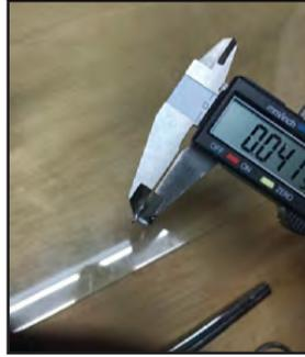
This will tell me how deep I need to drill through the plate. I will use a drill press with a forstner bit and set the stop depth
