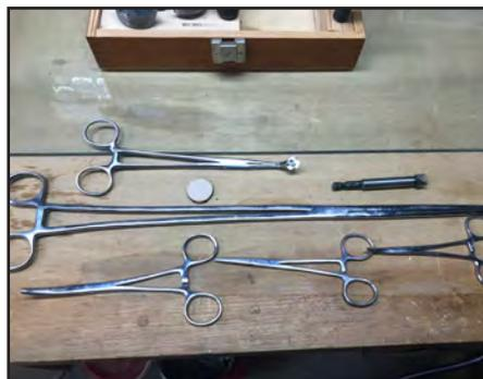
The nice thing about forceps is you can clamp them down and change angles of how it is held to get to those hard to reach areas. They clamp with enough force to really keep the blind nut secured until you release the handles on the forceps.
