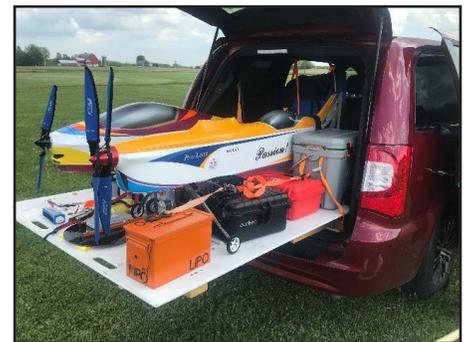
To use the slide, pull the two pins and pull the top sheet out about 5/8 of way, just enough so you can fold the table leg down and clear the van. (Mark the position so it is easily repeatable.) The side angles will hold the sheet up while you unfold the dining leg.
