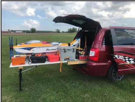
If you want even more storage, you can also use PVC tubing and build a frame that rests on top of the angle brackets. Lay some 1 1/2" insulating foam on top of the frame to create a shelf. With this shelf in place I have carried more than a dozen planes to an event including the 35%, a 25%, a Radian Pro, and the equipment needed for a weekend.
