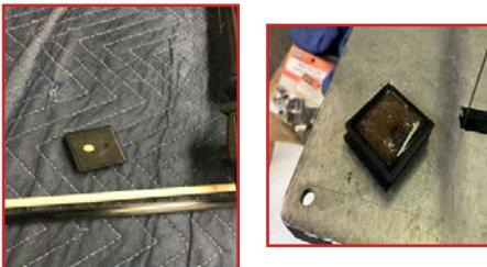
Here, the backplate is filled with epoxy and is set aside on my jigsaw. If you run the jigsaw all of the epoxy bubbles with float to the top of the piece and the epoxy is clear inside without bubbles.
