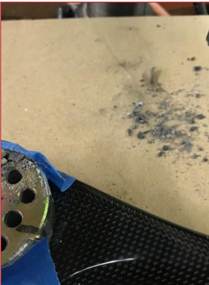
I generally use a small shop vacuum that has a filter to remove this from my drill press area. Once you have drilled all six holes, you should have a cleanly drilled prop. If you find your props split on the opposite side of the prop, use a spill board as I have pictured here and keep in mind you will have to sharpen drill bits more often (or replace) when drilling through carbon fiber.
