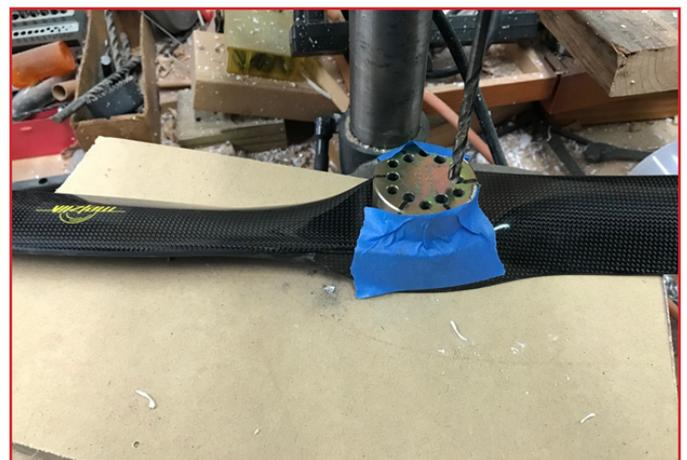
After the first hole is drilled, insert a dowel rod into the first hole. This helps keep the jig from turning on the face of the prop. Using the tape and dowel rod has helped me consistently drill props for years. Note that I use a spill board under my prop while on the drill press.
