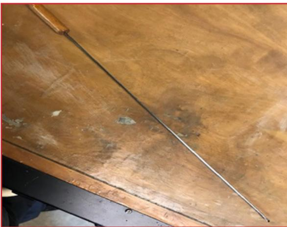
This driver is made from a 1/2" piece of dowel and a 2.5' piece of 1/8" music wire. I first cut a 3" piece of dowel and drill a 1/8" hole about 2.5" into dowel using a drill press. I also carve a notch on the opposite end of the drill hole. I use this notch to tell how far of a turn I'm adjusting my carbs.
