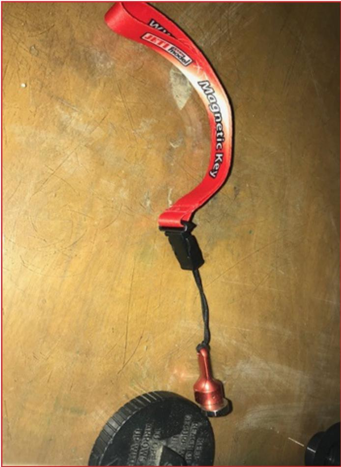
My last tip is for all of you JETI radio pilots out there that use magnetic switches. If your magnetic switch placement cannot be close to the exterior of your plane (i.e. in the canopy a 1/2" or so), you can place one of the neodymium magnets on your magnetic switch key (place magnet near the hole on the key) and you can significantly extend the reach of your switch key.
