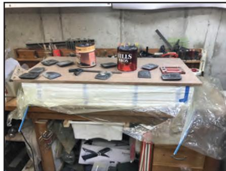
stick to vacuum bag material. Place paper towel down all seams of the parts so that any epoxy that wicks out will stick to the paper towel and not the bag. Hold paper towels in place with blue painter's tape. I generally will go through a whole roll of paper towels doing a 35-40% plane. The paper towel also does a good job of being breather material for the vacuum bagger so you have equal pressure throughout the part.
