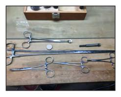
The nice thing about forceps is you can clamp them down and change angles of how it is held to get to those hard to reach areas. They clamp with enough force to really keep the blind nut secured until you release the handles on the forceps.
