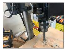
on my drill press. I will generally use thick CA to glue the new disc plate to the inside of the plane. Do not put glue in the center of the disk as this could get into the threads of the blind nut.
