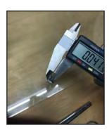
This will tell me how deep I need to drill through the plate. I will use a drill press with a forstner bit and set the stop depth
