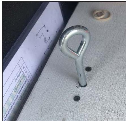
Next you will need a stop to hold the top sheet in position when driving. I cut two pieces of 2x4 wood, one for each side, that matched the spacing between the top and bottom sheets. These I screwed to the bottom sheet about 4” from the table end and 3” from each side. Then I drilled a 1/2” hole through the two sheets and wood blocks. Then used a long bolt as a pin to lock the top sheet in place.
